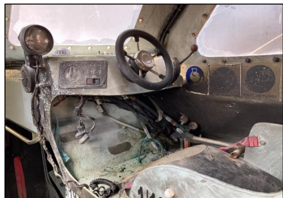
Figure 5: Control panel damage
