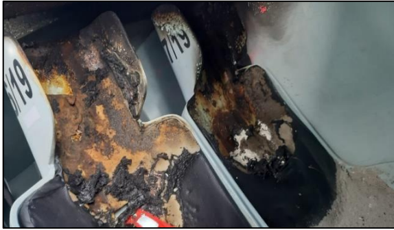
Figure 7: Fire / smoke damage to the seat cushions
