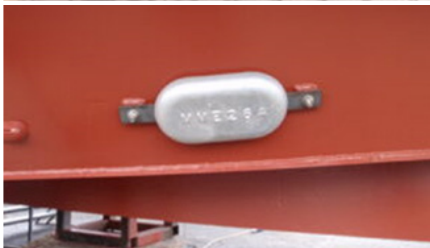
Narrowboat anodes can be fitted as either welded or bolt on
