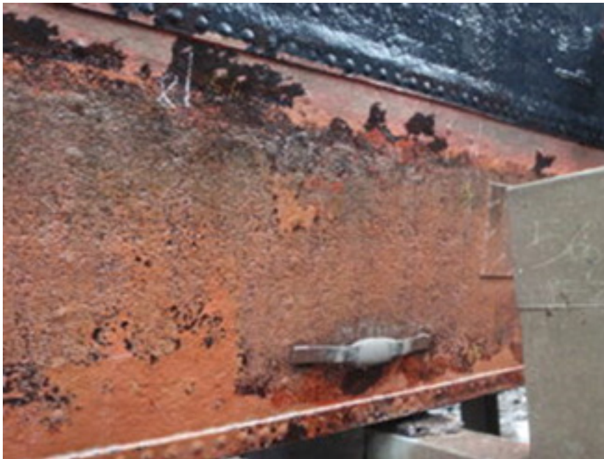
Fully wasted zinc anode – 'well sucked lollipop'
