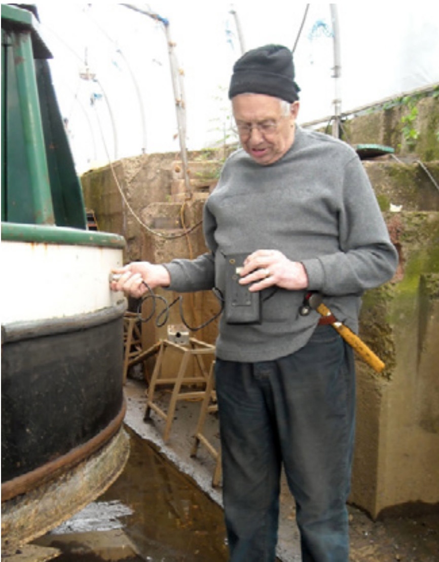
Taking UTS Measurements on a Narrowboat in the Dry Dock at Enfield.
