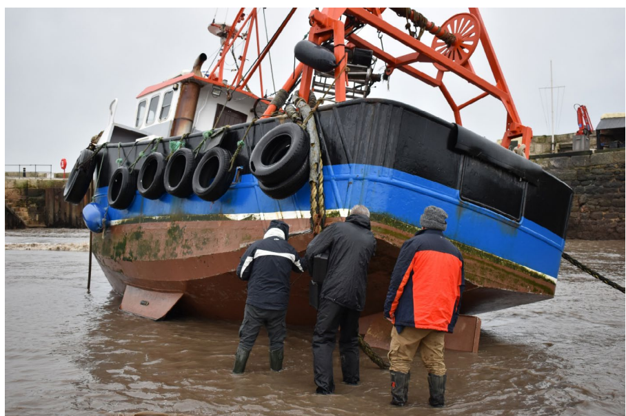
Jon Sharland oversees ultra-sonic thickness measuring on a steel hull in the harbour
