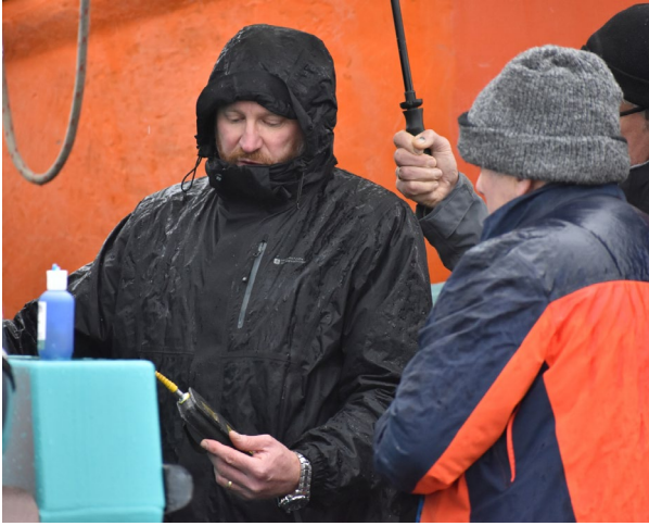
Jon Sharland and students thickness testing a GRP hull on the hard
